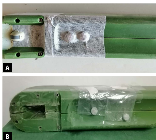
Figure 2: The iButtons were placed inside the PAP next to the aspiration line (A), and on the outside (B) of the PAP in order to record the temperature the oocytes will be exposed to and the rhinoceros' rectal temperature, respectively.
